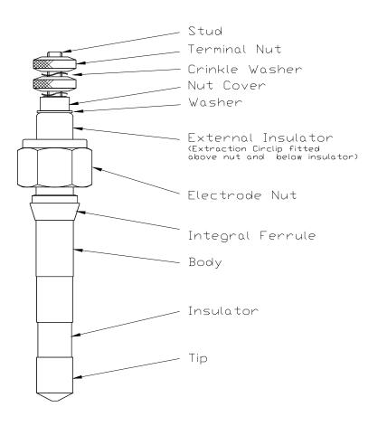
Figure 4.2 - High pressure electrode
